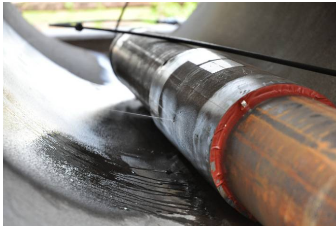
Figure 38: Leakage of specimen no. 2
