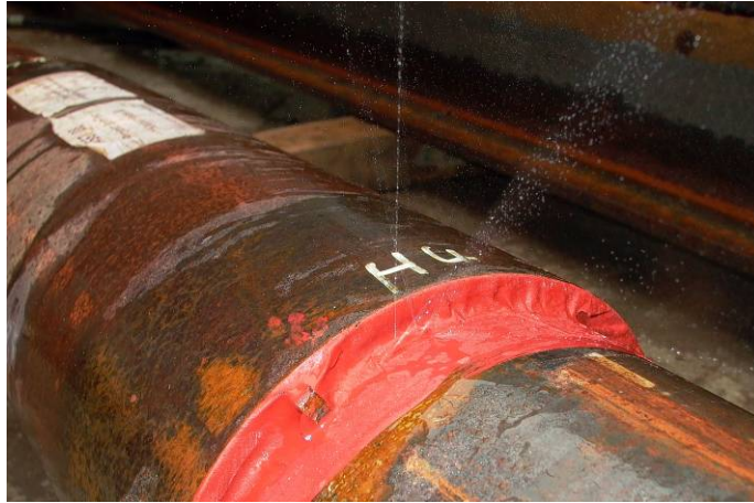
Figure 40: Second leakage of specimen no. 2
