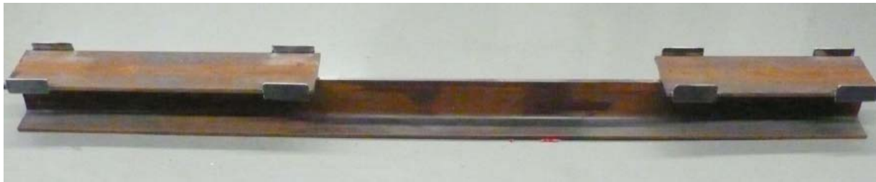
Figure 30: Device for centring and aligning steel pipes for adhesively bonding
