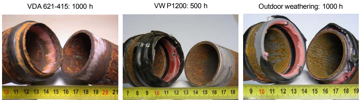
Figure 11: Appearances of fracture of small scale pipe specimens aged under VDA 621-415, VW P1200 and outdoor-weathering
