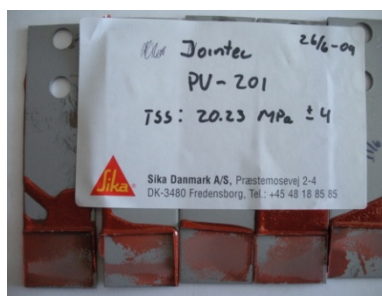
Figure 16: lap-shear specimens of PU-201 one side
