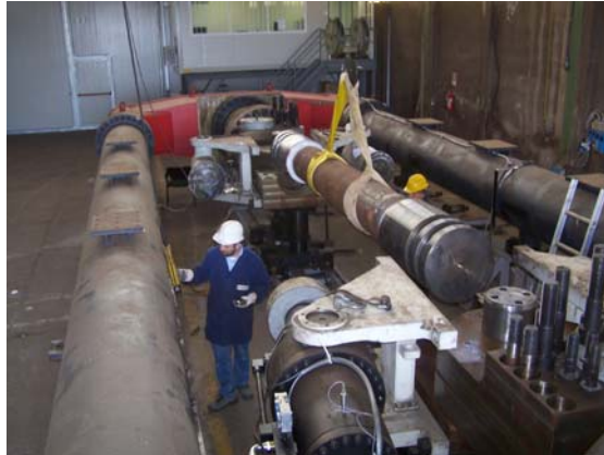
Figure 58: Trial specimen loaded into the full scale test frame
