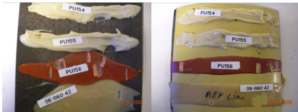
Figure 14: Evaluation of four adhesives the top one is PU-155, then PU-154 the red one is PU156 and the last one is 06-060-42 on epoxy coated surface and un-treated steel respectively
