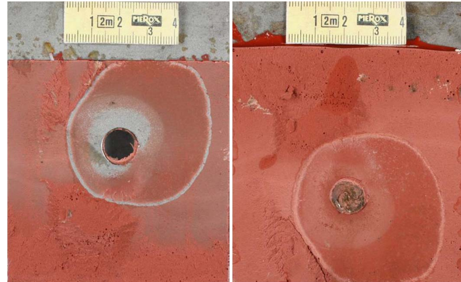
test 2: no leak at 300 bar
