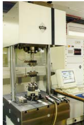
Magnetic pulse resonance testing facilities frequencies up to 300 Hz
