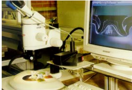
Digital-optical facility for rivet joints quality control
