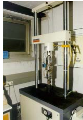
Magnetic pulse resonance testing facilities frequencies up to 300 Hz
