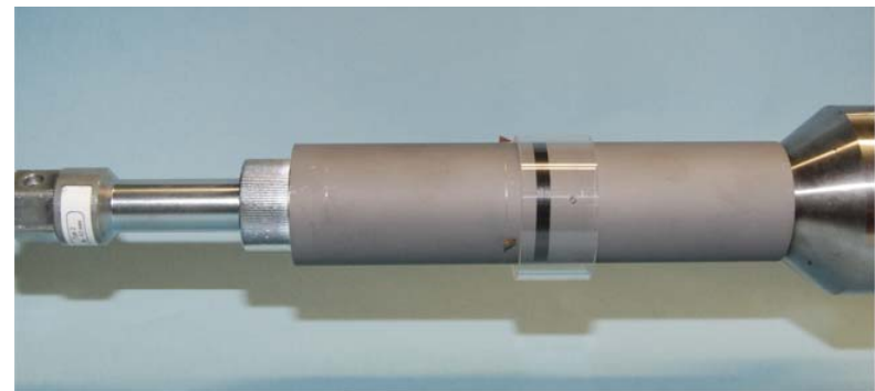
step 4a: defining the glue line using steel wedges
