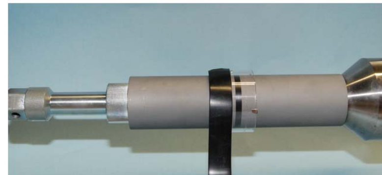
step 5a: application of shrinking material; tacking of the shrinking tube
