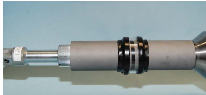
step 6: specimen prepared for adhesive injection
