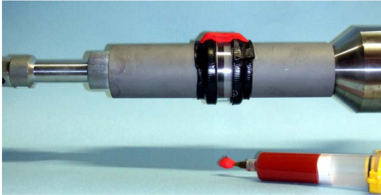
step 6a: sealing of the upper hole
