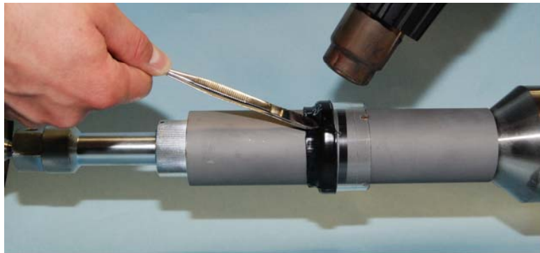
step 5d: sealing the overlap of the shrinking material
